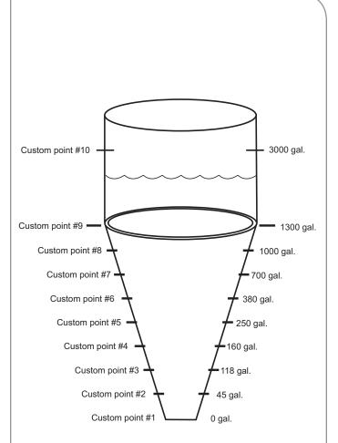
In the LEVEL/VOLUME INPUT menu (see page 40), if SHAPE is set to HORIZ CYLINDER, RECTANGLE or CUSTOM, the tank shape can be defined with the following screens:
