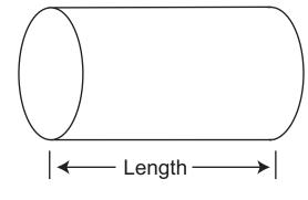
Pressure to level conversion:  $Level = P \div (SG \times D)$ where P = Pressure SG = Specific Gravity of fluid D = Density of water With pressure in psi:
