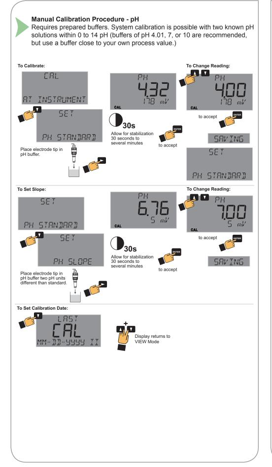
Single-point calibration sets STANDARD only; Signet recommends a two-point calibration to set SLOPE in addition to STANDARD.
