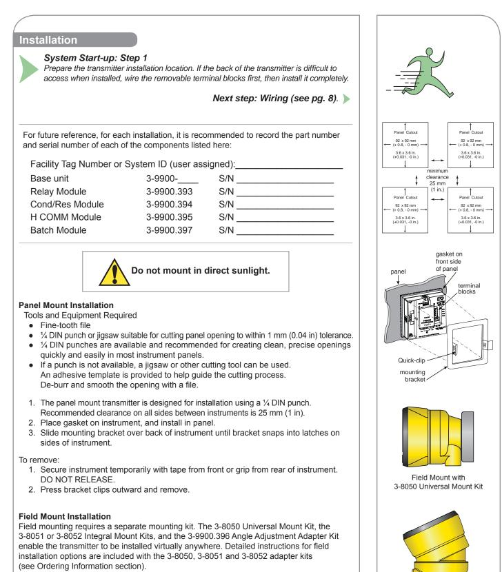
For Field Mount installations with a Cond/Res Module, the 3-9900.396 Angle Adjustment Adapter is required along with a 3-8050 or 3-8052 adapter kit to allow for sufficient clearance for the wiring.
